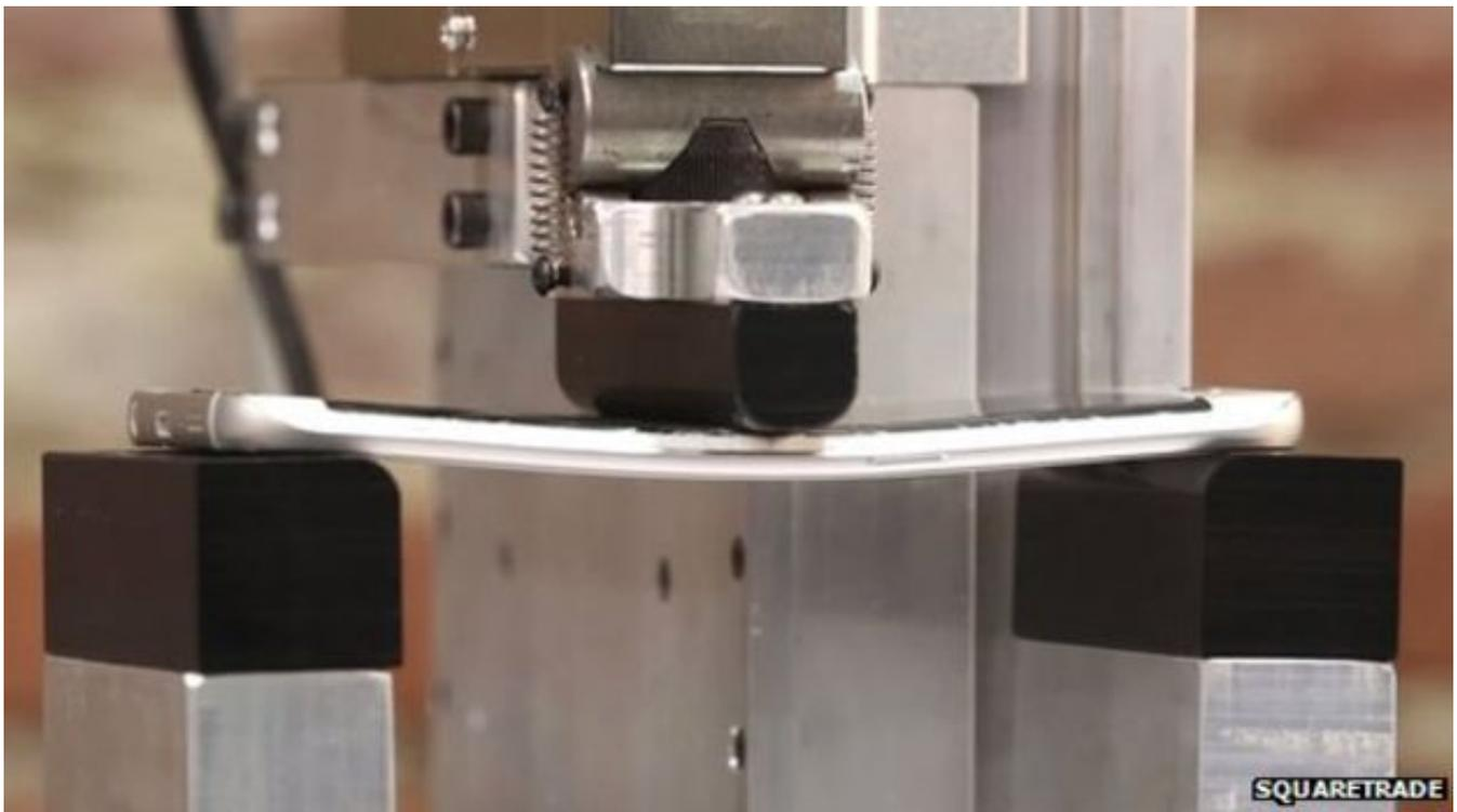
The test found that the S6 Edge's screen cracked at the same point that the phone bent
